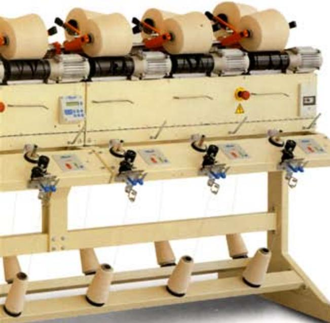
**CONE TO CONE WINDERS Mod. SES** with one inverter each modulus
